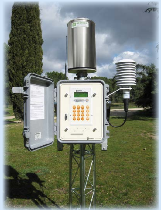
RAINALERT / HYDROMET Station with METEODATA Unit
