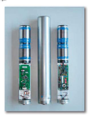
The GammaMETER RS04 consists on a proportional counter tube (type NPGD02). A large number of these counter tubes have been in operation in several European countries for many years and have set a new worldwide environmental surveillance standard. This specific model is unique as it is the only one able to cover a 9-decade measuring range with a single detector.
