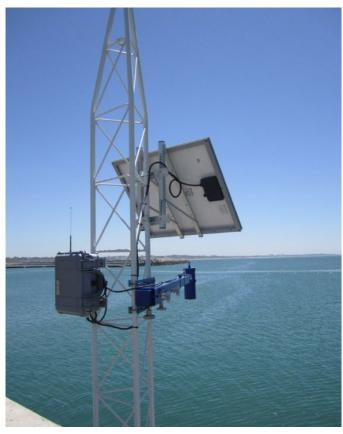
RADAR-6115 water level sensor assembly on extensible-retractile support arm mounted on a tower
