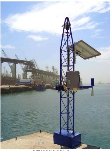
**DATAMAR** RADAR Tide Gauge with RADAR-6135 water level sensor mounted on the air
