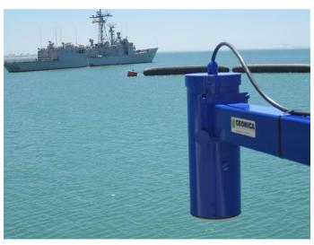
Water Level Sensor Model RADAR-6115
