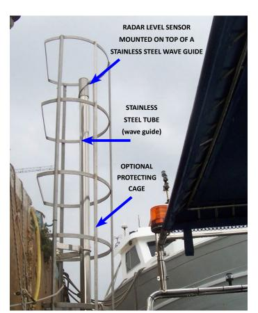
RADAR level sensor assembly on stainless steel tube
