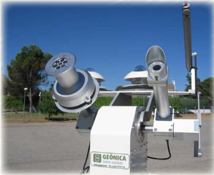
Pyrheliometer, Pyranometer and Solar Spectral Irradiance Sensor mounted on Suntracker-3000
