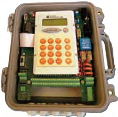
METEODATA/HYDRODATA Datalogger with integrated comms (3G/GPRS, Line, Radio or Satellite)
